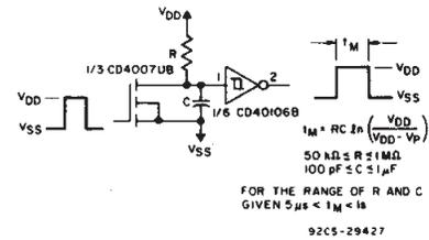
Fig. 17 - Monostable multivibrator.
