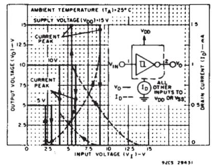
Fig. 8 - Typical current and voltage transfer characteristics.
