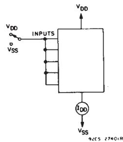
Fig. 19 - Quiescent device current test circuit.
