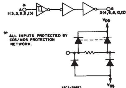
Fig.1 – Logic diagram (1 of 6 Schmitt triggers).
